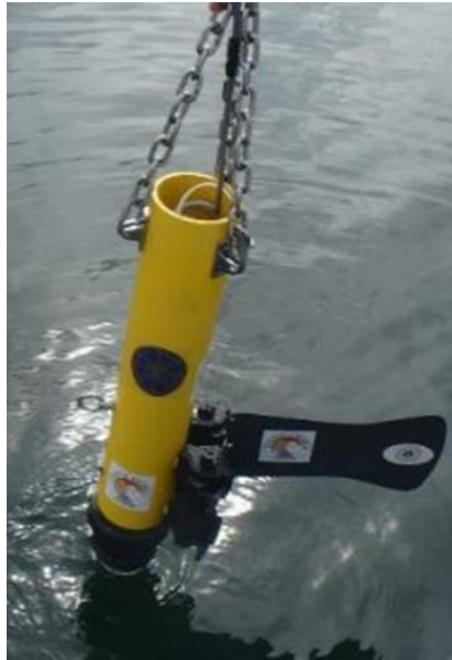
Figure 2. MMA 2016 underwater video HD camera system.
